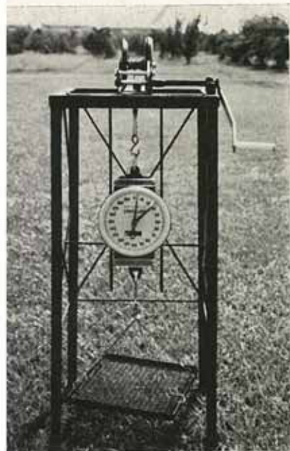
Figure 3: Apparatus for measuring sod rooting strength.
